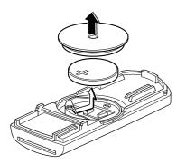
5. Insert a new battery with the positive pole facing up, and then cover the battery with the battery cap.
